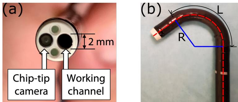
Figure 3. Pentax VNL-1570STK video laryngoscope: (a) This flexible endoscope includes a chip-tip camera and a 2 mm side working channel; (b) View of the endoscope showing constant-curvature bending, with  $R$  being the (variable) bending radius and  $L = 25.7$  mm being the length of the bending section.
